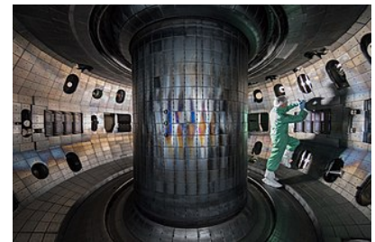
Figure 3.8: Experimental tokamak fusion reactor DIII-D. Figure from commons.wikimedia.org under license CC BY-SA 4.0 .
