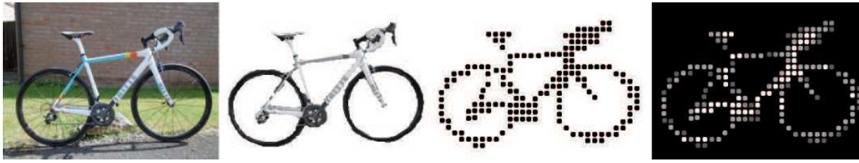
Figure 1.8: An example of image processing in the Argus II retinal implant (Bloch and da Cruz, 2019). The image first undergoes edge detection and is converted to greyscale. It is then transformed by circular binarisation into a black-and-white pixelated format. Finally, the image is inverted, with the addition of four greyscale levels.
