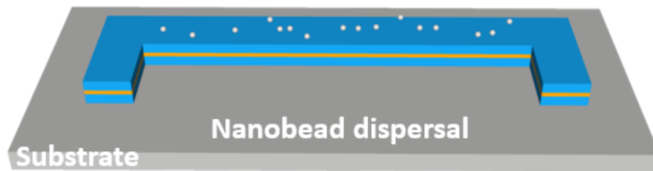
Figure 6.4. Schematic presentation of the nanobead process Step-I i.e., nanobead dispersal. The dark gray colored area represents the substrate ( \text{Si}|\text{SiO}_x ), while the layers with sky-blue color represent the FM electrodes (top and bottom). The sandwiched dark yellow colored layer represents the organic molecular layer (or the spacer layer). The white spherical-shaped objects on the top surface (capping layer) of the hybrid trilayer stacks are the silica nanobeads, that will be used as a shadow mask to define the cross-section of the vertical nanopillars during the \text{Ar}^+ -ion etching step (Step-II).[33]
