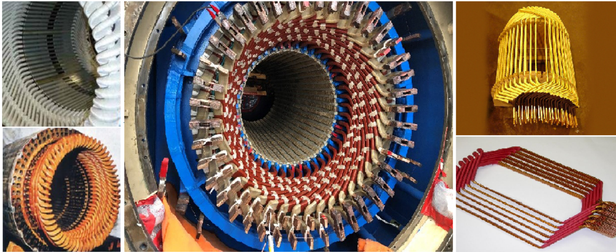
Figure 3.18: Generator's with form-wound coils
