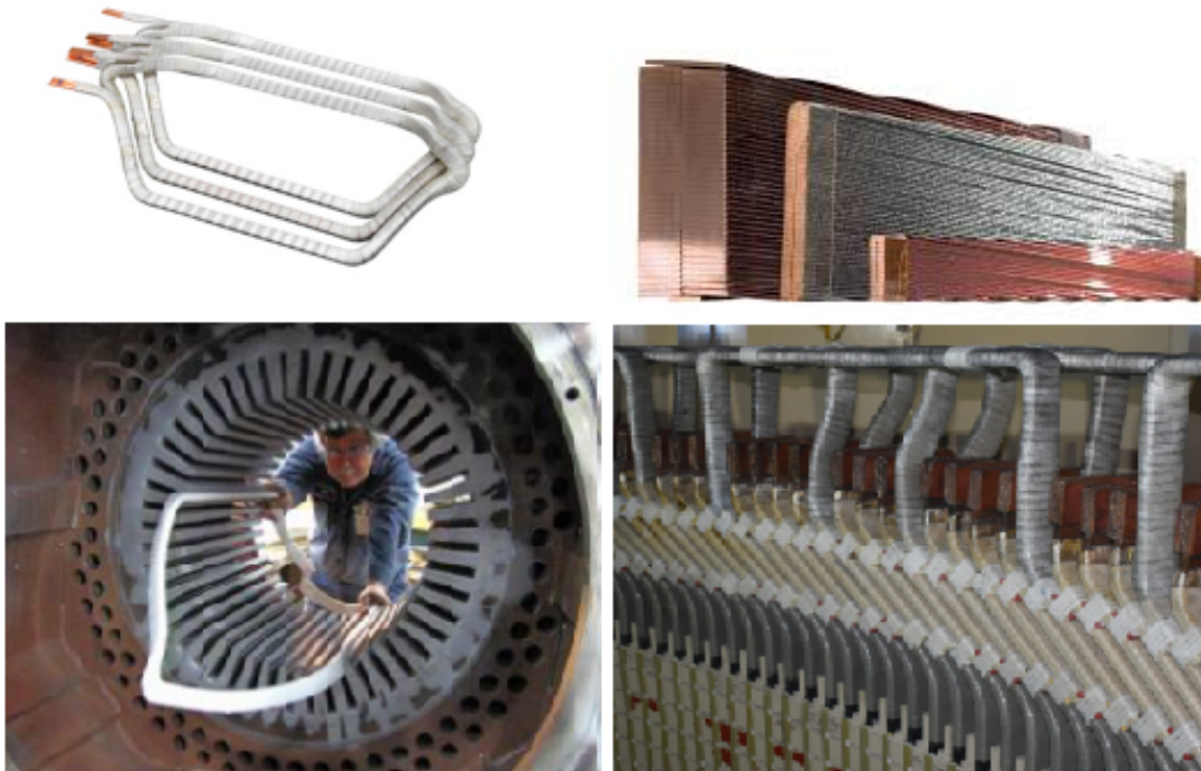
Figure 3.20: Multi-turn pre-formed stator coils (left) and single-turn stator bars (right)
