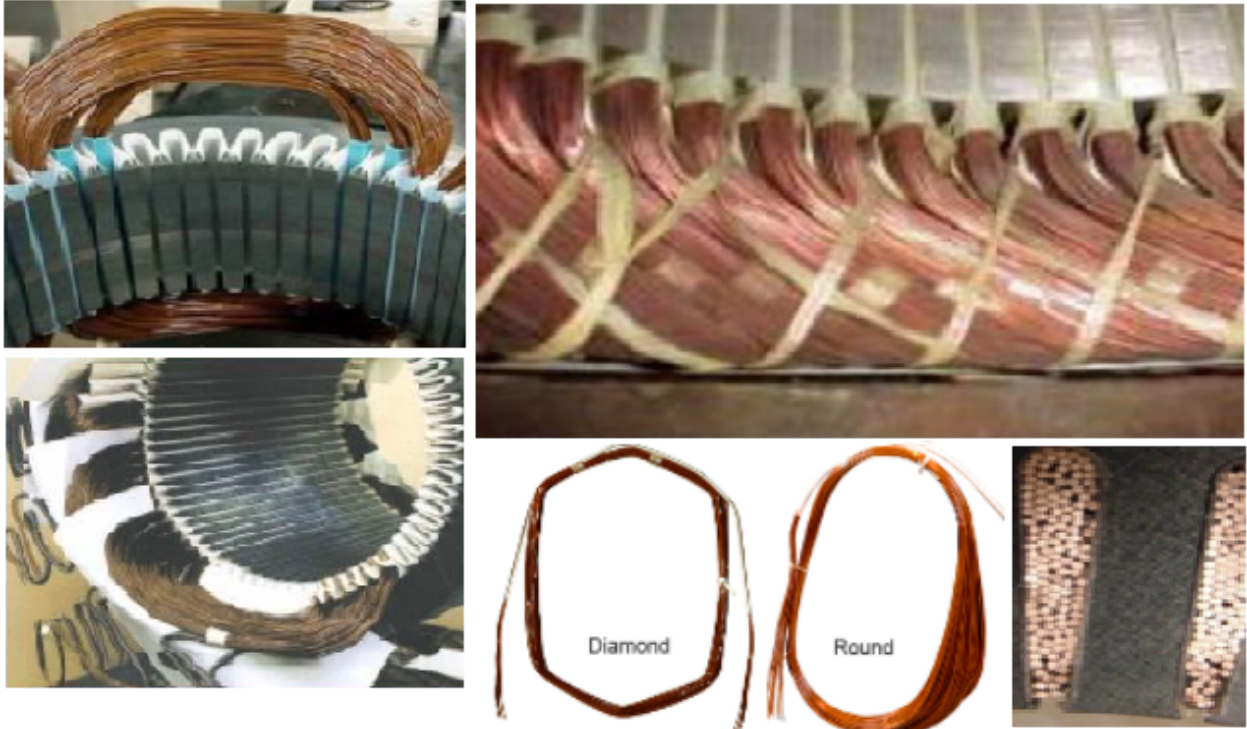
Figure 3.19: Generator's with random-wound coils
