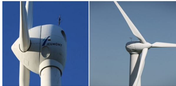
Figure 2.12: Jeumont J48/750 direct-drive AFPMSG wind turbine
