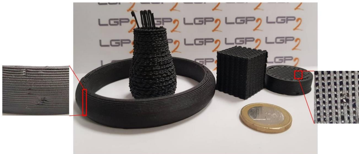
Figure 5-32: A selection of printed objects with a zoom of broken filament on the right and visible z-seam of the left.
