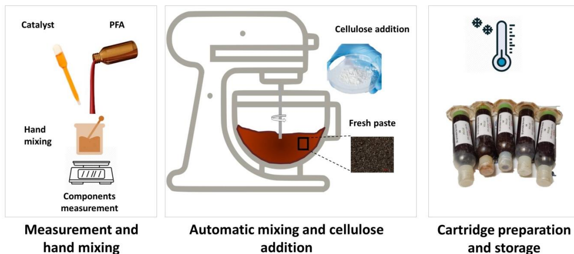
Figure 2-5: Illustration of the paste preparation method.
