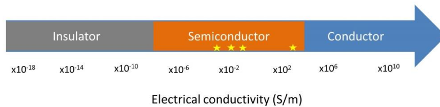
Figure 4-37: Materials classification based on their electrical conductivity levels and the positioning of biocomposite developed in this work.
