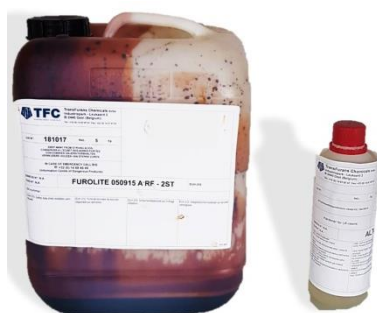
Figure 2-4: Photos of the used viscous PFA resin (left) and the catalyst (right).
