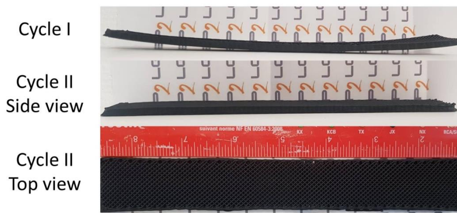
Figure 5-33: Arching of a printed thin bar when changing the thermal curing cycle.
