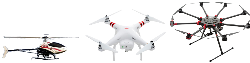
Figure 2.3.: Depiction of the three drones used in simulations. From left to right: The Vario helicopter, DJI's Phantom2, a quadcopter, and S1000+, an octocopter. Scale is not respected.
