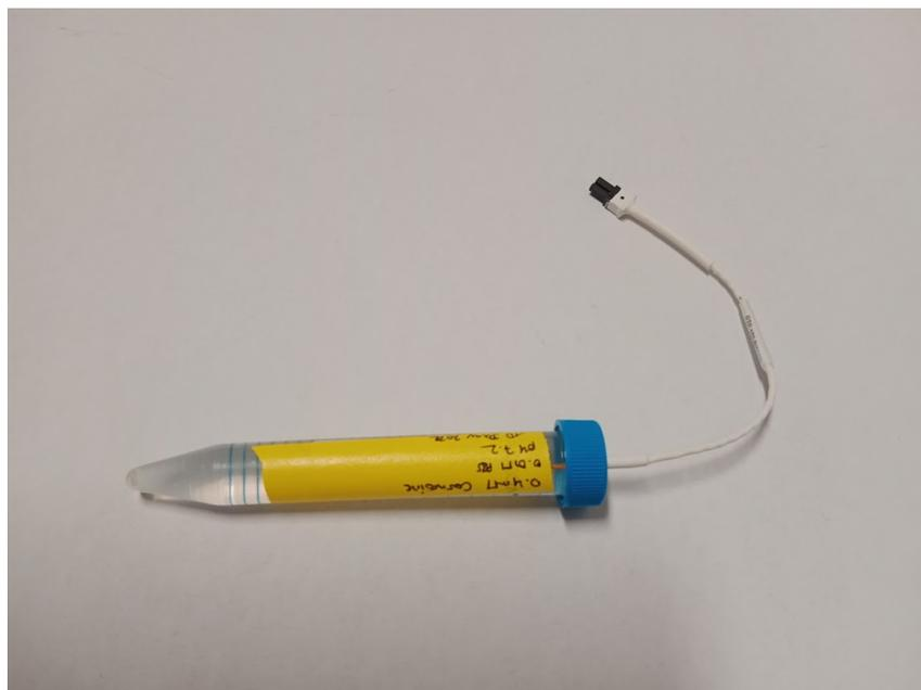
Figure 2.7: Temperature probe inserted in a phantom
