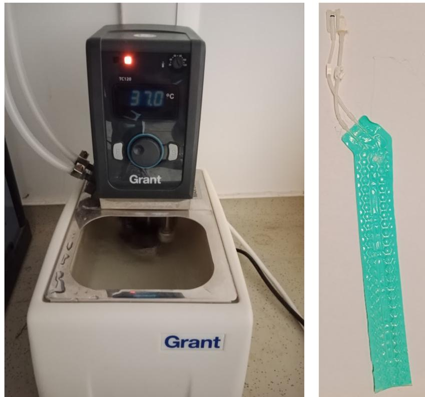
Figure 2.11: Heating system : water bath with an adjustable temperature (left) connected to a blanket (right) wrapped around the animal (or the sample)
