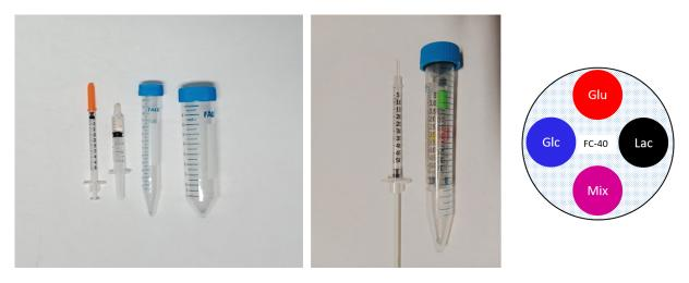
Figure 2.6: Phantom containers. Left: 0.5 mL syringe, 2.5 mL plastic syringe, 15 mL Falcon tube, 50 mL Falcon tubes. Middle: Example of a 0.5 mL syringe next to the 15 mL Falcon tube enclosing the four 0.5 mL syringes. Right: Schematic representation of the 4-compartment phantom, the four syringes are surrounded by FC-40.
