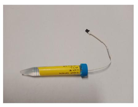
Figure 2.7: Temperature probe inserted in a phantom
