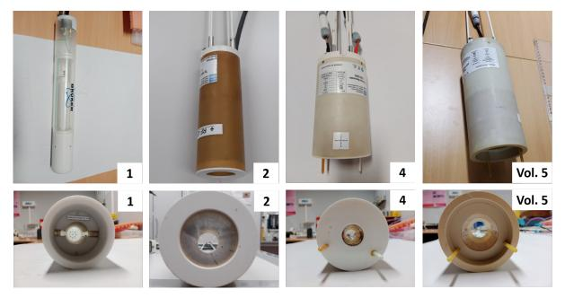
Figure 2.3: View from above (top) and axial view (bottom) of the volume coils : coil  $n^{\circ}1$ , coil  $n^{\circ}2$ , coil  $n^{\circ}4$  and volume coil from combination  $n^{\circ}5$
