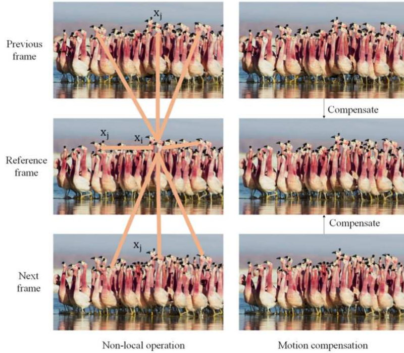
Figure 2.6: Differences of non-local operation and explicit motion compensation. Non-local operation tries to obtain the response at position x_i by computing the weighted average of relationships of all possible positions x_j [133]. Figure taken from [150].
