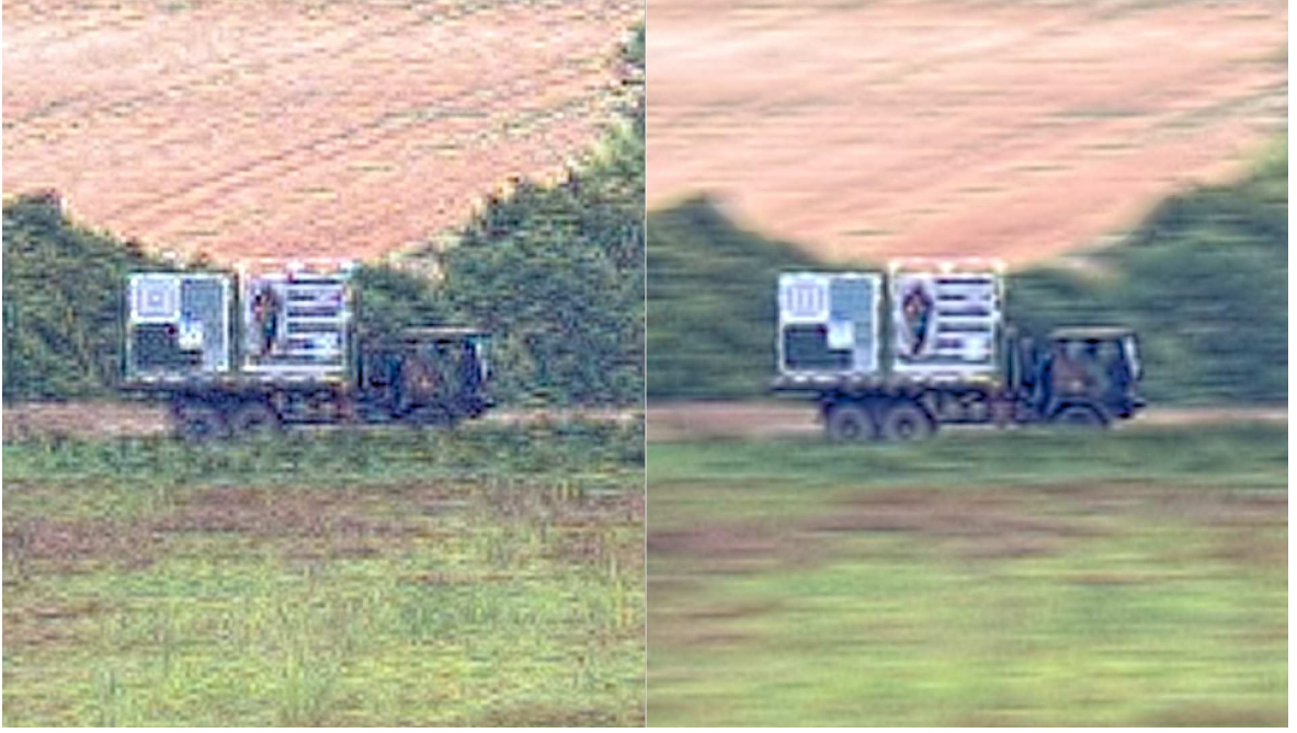
Figure 2.11: Classical VSR with a mobile object. Left: input degraded frame. Right: the corresponding super-resolved frame.
