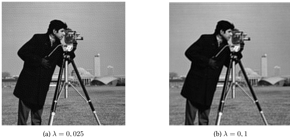
Figure 1.3: Deconvolution based on Tikhonov filtering, with L = I . \lambda denotes the regularization parameter. The noise is white, additive and Gaussian with standard deviation \sigma = 1 . The blur kernel described in Fig. 1.1 has been used.
