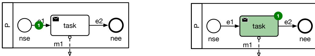
Figure 4.19: Starting Behaviour of a Send Task Activity. Before (left) and after (right) application of the St rule.
