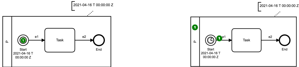
Figure 5.1: Completing Behaviour of a Timer Start Event (Date). Before (left) and after (right) application of the Ct rule.
