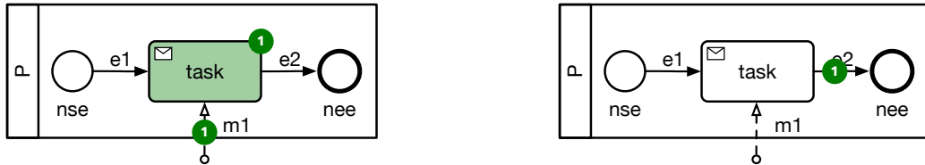
Figure 4.21: Completing Behaviour of a Receive Task Activity. Before (left) and after (right) application of the Ct rule.
