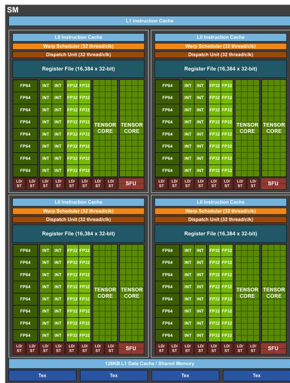
FIGURE 3.17 – Volta Streaming Multiprocessor. (Source : Volta-V100 Whitepaper, NVIDIA.)
