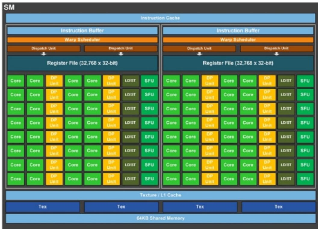
FIGURE 3.16 – Pascal Streaming Multiprocessor. (Source : Pascal-GP100 Whitepaper, NVIDIA.)
