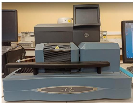
**Figure 2-7.** *SDT Q600 V20.9 Build 20 Thermogravimetric Analyzer.*
