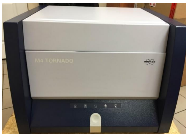
Figure 2-4. Micro-X-ray Fluorescence spectrometer M4 TORNADO (Bruker).
