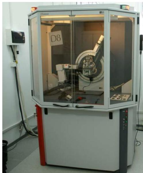
**Figure 2-3.** Bruker AXS D8 diffractometer.
