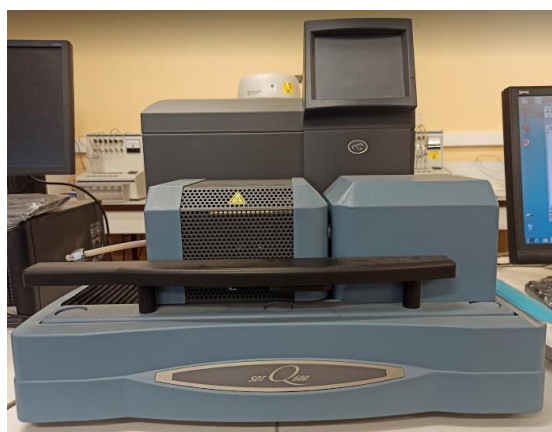
Figure 2-7. SDT Q600 V20.9 Build 20 Thermogravimetric Analyzer.
