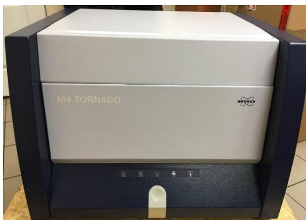
**Figure 2-4.** *Micro-X-ray Fluorescence spectrometer M4 TORNADO (Bruker).*
