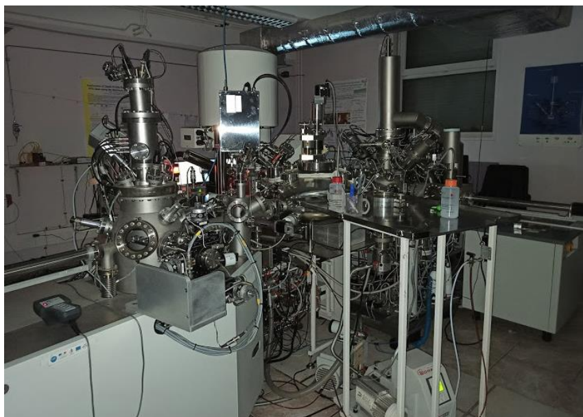
Figure 2-8. X-Ray Photoelectron Spectra (XPS) Kratos AXIS UltraDLD spectrometer.
