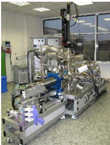
**Figure 2-9.** *Near Ambient Pressure X-Ray Photoelectron Spectroscopy at Charles University.*
