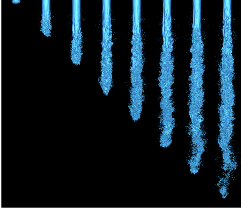
Figure 1.19: Turbulent atomization of a liquid Diesel jet with the original Accurate Conservative Level Set (ACLS) method (2008). Reprinted from [31].
