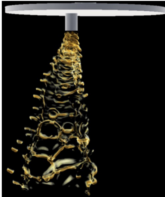
Figure 6.12: Volume rendering of the atomizing jet issued from a low-pressure compound nozzle.
