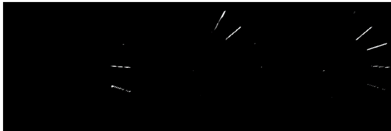
Figure 7.11: Reconstructed needles maps obtained with the DTV decomposition method on Phantom (B). From left to right: x_{\Omega_1} ( \theta_1 = 107.5^\circ ), x_{\Omega_2} ( \theta_2 = 27.5^\circ ), x_{\Omega_3} ( \theta_3 = 72.5^\circ ).
