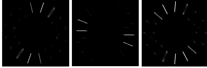
Figure 7.14: Reconstructed needle maps of Phantom (B) for \theta \in [-35^\circ, 15^\circ] with a 1D regularization. From left to right: component of direction \theta_1 , component of direction \theta_2 , sum of rotated components.
