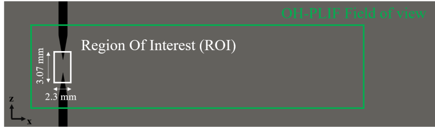
Figure 5.13: Schematic representation of the OH analysis regions. The green rectangle indicates the field of view of the OH-PLIF. The white rectangle indicates the Region Of Interest (ROI) in the discharge zone.
