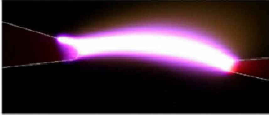
Figure 2.2: Digital camera image of a spark plasma discharge. Extracted from (Pai et al. (2008)).
