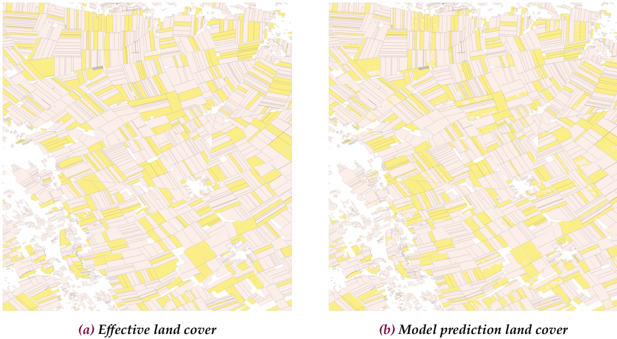
Figure 2.20: Visualization of observed and predicted crop rotation of soft winter wheat parcels under the 2d\text{-CNN-TT}_{\text{Temporal-Conv}} experiment in the studied sub-area of France-East zone over the campaign 2017/2018. Yellow pixels are those of soft winter wheat crop, the remaining pixels represent other crops.
