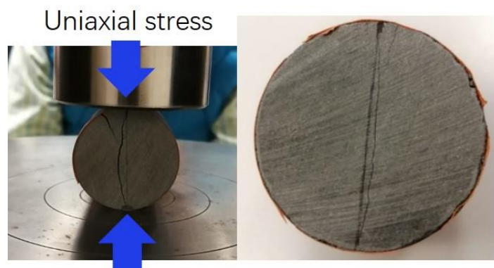
Figure 4.2. Photograph of a Brazilian test (left) and the resulting diametral macro-crack (right)
