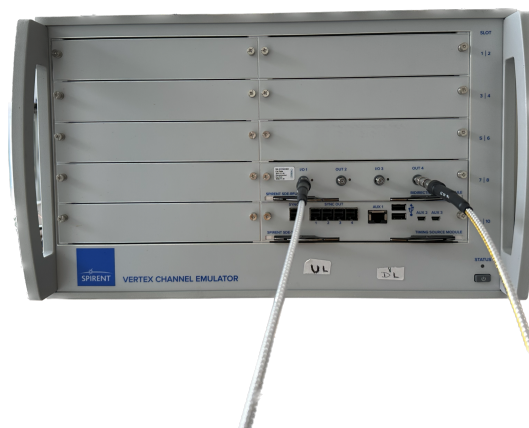
Figure 4.24: Spirent Vertex Channel Emulator
