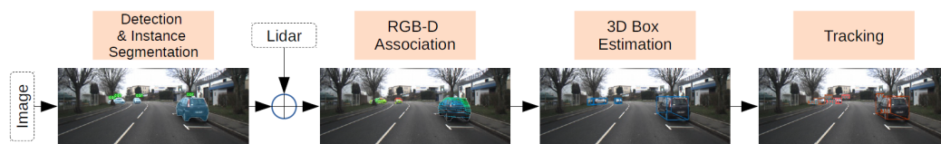
FIGURE 3.5: Pipeline for 3D object detection. Objects are detected in the images from the cameras. Later, LiDAR data is included to infer the geometrical properties of the objects. Finally, all the detections are merged, and a tracking stage adds temporal consistency across consecutive frames [318]
