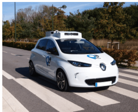
FIGURE 3.2: Renault ZOE automated vehicle
