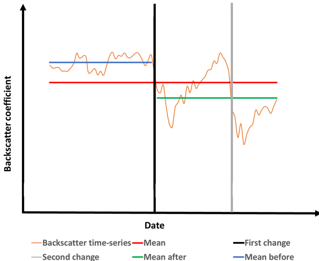
Figure V.3: Application of ReCuSum on a backscatter coefficient time-series. The vertical black line is the date of change found by the first iteration of the CuSum, the vertical grey line is the date of change found by the second iteration of the CuSum. The backscatter time-series is symbolized by an orange line, and its mean is symbolized in red (mean over the entire time-series), blue (mean before the first change) and green (mean after the first change).
