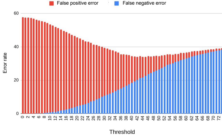
Figure VI.6 – Error rates of recurrent speaker detection on the DEV part of the ALLIES dataset with SINCNET within-show baseline and VAD segmentation. For each value of the threshold, the bar plot represents the percentage of false positive and false negative errors in red and blue respectively.
