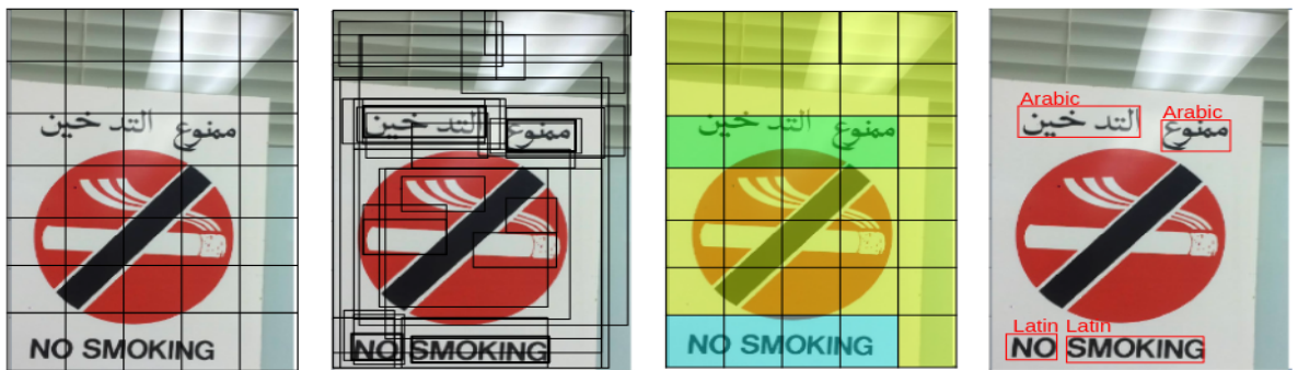
Figure 5.2: From left to right: The input image presented to the network in its full size is divided into S \times S grid. Secondly, for each grid cell we predict the BB with the CNN. Third the probability for the box to be within a specific class. Last image presents the final output after NMS.
