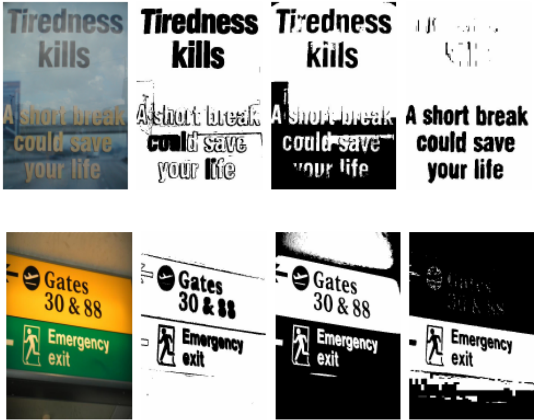
Figure 4.2: Multi-level binarization results of two test images. From left-to-right images are shown followed by their binarization results for: smooth/non-smooth binarization, adaptive thresholding binarization on the original image and on the complement of Hue channel. Note that some text components appear in only one of the binary images.
