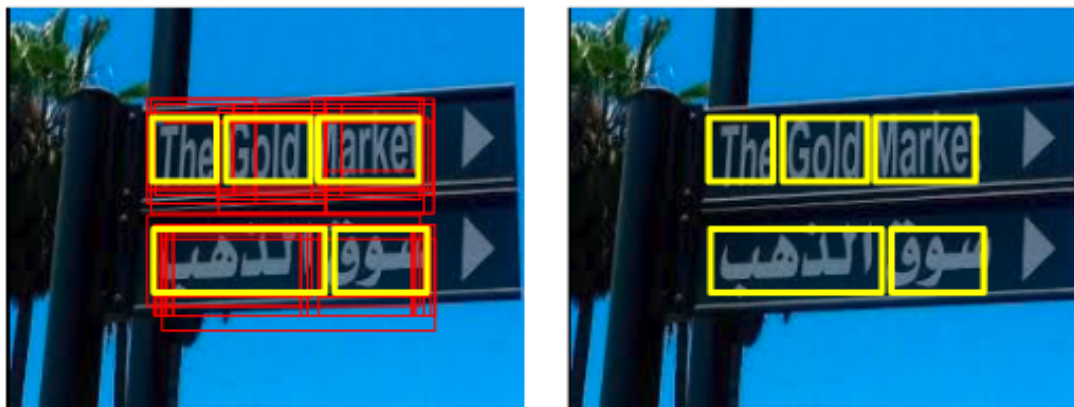
Figure 5.4: The use of Non-Maximum Suppression to fix the multiple detection of the same zone of text. The first figure presents the output of the CNN. The second image presents the final detection result after the NMS step, where one box per word is chosen.
