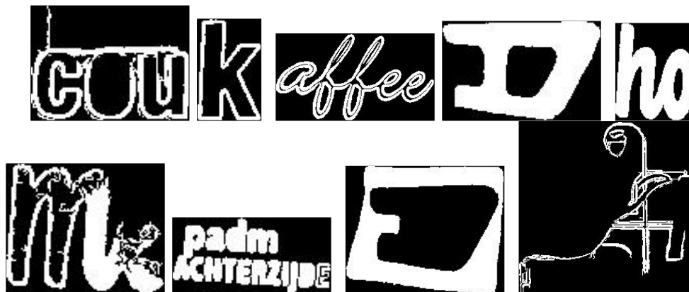
Figure 4.4: Samples of extracted CCs from different binarizations of different images. The components are of different sizes, orientations and shapes, and of variable types: letters, groups of letters and varying non-text components.
