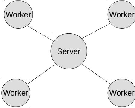
FIGURE 6. Centralized distributed system
