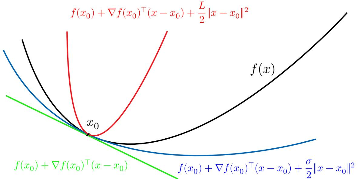
FIGURE 1. Graphical illustration of the quadratic upper-bound and lower bound provided respectively by  $L$ -smoothness (in red) and  $\sigma$ -strong-convexity (in blue) at point a  $x_0$  for a function  $f$ .
