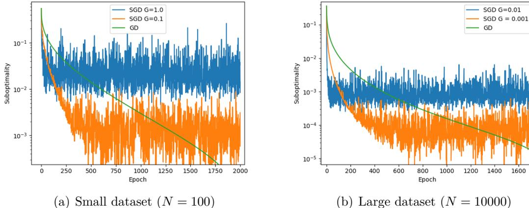
FIGURE 3. Comparison between deterministic and stochastic gradient descent on the LibSVM *a9a* dataset, for a regularization  $\lambda = 10^{-3}$ . SGD was run with step size  $\eta = G/L$ . We see that SGD decreases the error rapidly, but quickly saturates to mean error level that depends on  $G$ .
