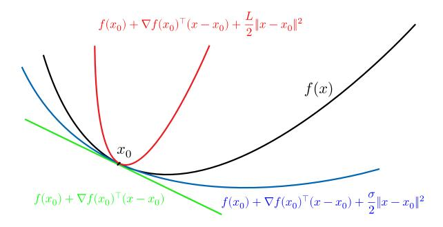
FIGURE 1. Graphical illustration of the quadratic upper-bound and lower bound provided respectively by L-smoothness (in red) and  $\sigma$ -strong-convexity (in blue) at point a  $x_0$  for a function f.
