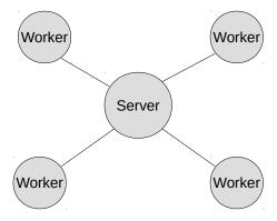
Figure 6. Centralized distributed system
