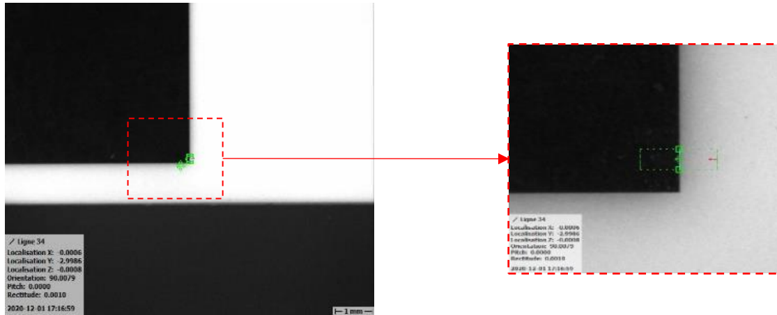
Figure III.16 Example of the process of extracting points for vertical line using black-to-white threshold of 125
