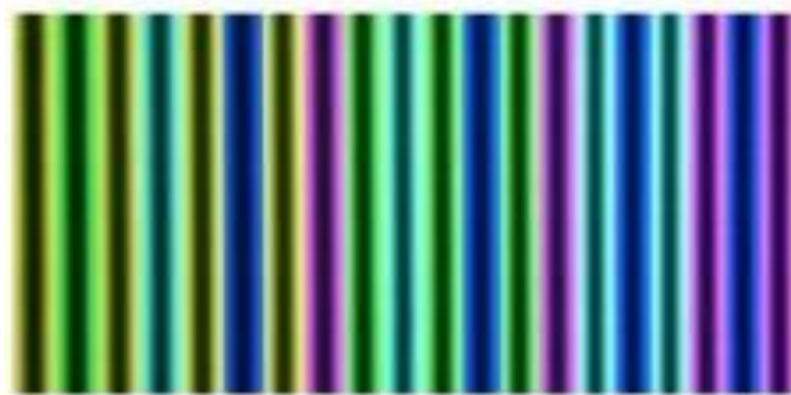
Figure A.3 Coloured stripe coding for 3D reconstruction using structured light systems
