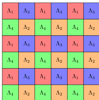
(b) Lattice model: every block is considered dependent only with its direct neighbouring blocks. This induces four sets of blocks, called lattices, \Lambda_1, \Lambda_2, \Lambda_3, \Lambda_4 where each block in a given set is independent of every other block in the same set.
