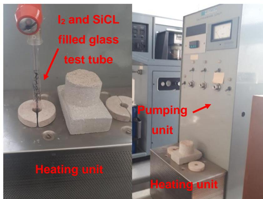
**Figure 3.3** Adapted BET heating and pumping unit used for the iodine annealing of the silicon clathrates films.
