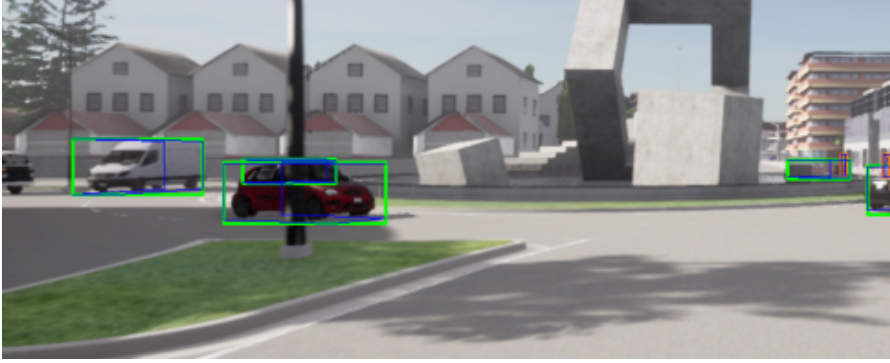
Figure 3.5: Example of a bounding box that should be deleted but is not because it belongs to the same class as the occluding object.
