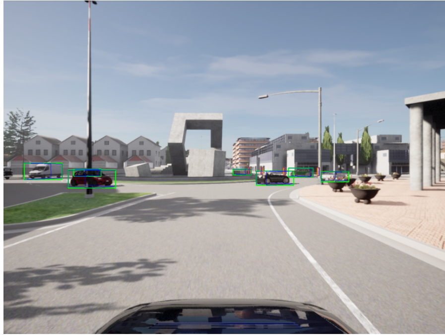
Figure 3.2: Bounding boxes for cars and pedestrians with their two lower points on the ground as given from our Dataset built from CARLA. Green boxes represent the 2D bounding boxes extracted from the 3D bounding boxes given by the simulator.
