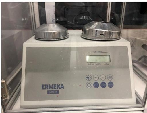
Fig. 2.13 Picture of the tapped density tester (SVM22, Erweka GmbH, Germany).
