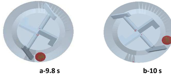
Fig.6.20 Snapshot of  $\gamma\text{-Al}_2\text{O}_3$  (1.0 mm in diameter, green in color) and  $\text{TiO}_2$  (0.1 mm in diameter, red in color) particles in picomix when the interfacial energy of  $\gamma\text{-Al}_2\text{O}_3\text{-TiO}_2$  is  $20 \text{ J/m}^2$  at 9.8-10 s of modeling time.
