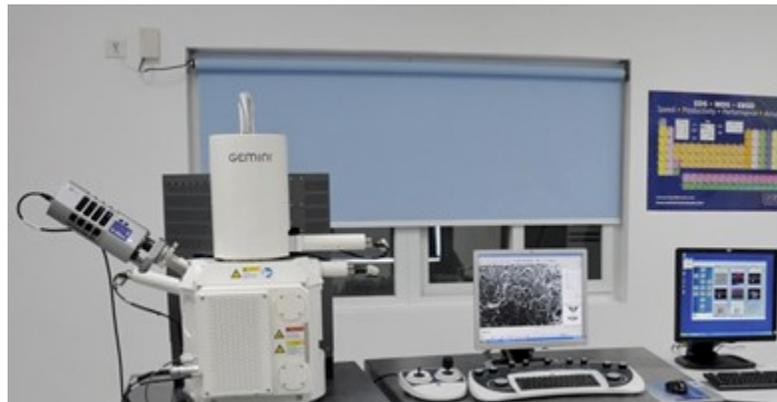
Fig. 2.12 Scanning electron microscope (Hitachi Ltd.).
