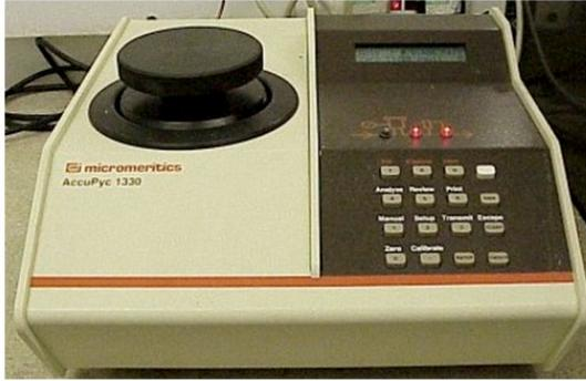
Fig. 2.11 The AccuPyc1330 Pycnometer (Micromeritics Instrument Corp.).
