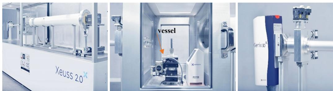
Fig. 2.8 Xeuss 2.0 SAXS instrument: a. the whole device; b. put sample part; c. detector.
