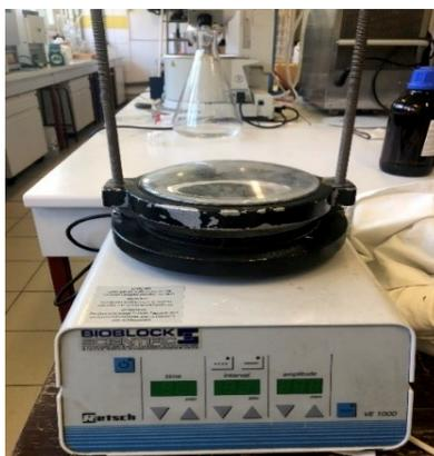
Fig. 4.5 The photo of sieve shaker (Retsch, France)
