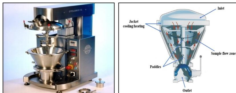
Fig.1.9 Photo (a) and schematic (b) of a Hosokawa Cyclomix [104, 105, 126].
