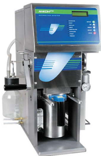
Figure I-38. Ankom XT15 extractor.
