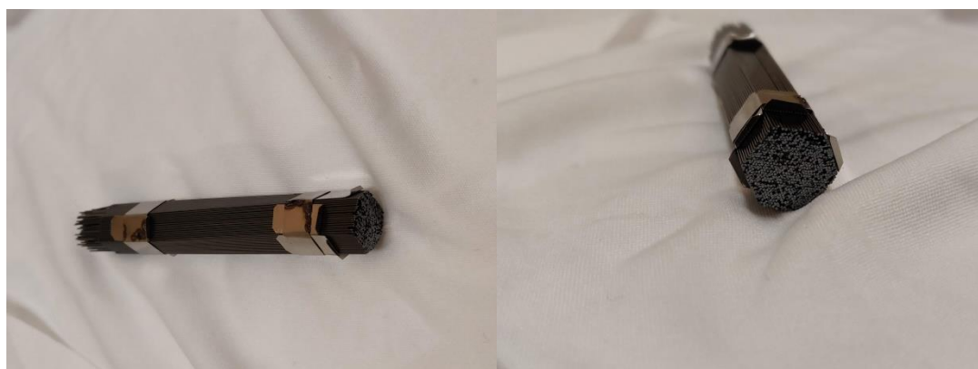
Figure 3.29 Stacked preform for fabrication of the graded-index fiber
