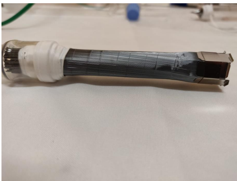
Figure 3.31 partially collapsed preform
