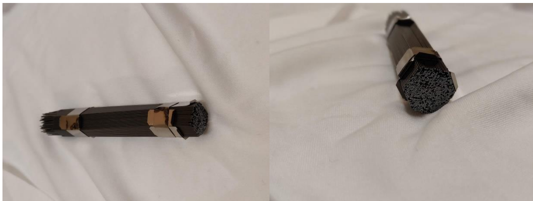
Figure 3.29 Stacked preform for fabrication of the graded-index fiber
