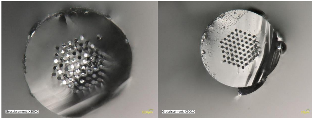
Figure 3.42 The images of the cross section of the PCF filled with TAS glass at the position of (left) 5mm and (right) 10mm to the bottom of the fiber
