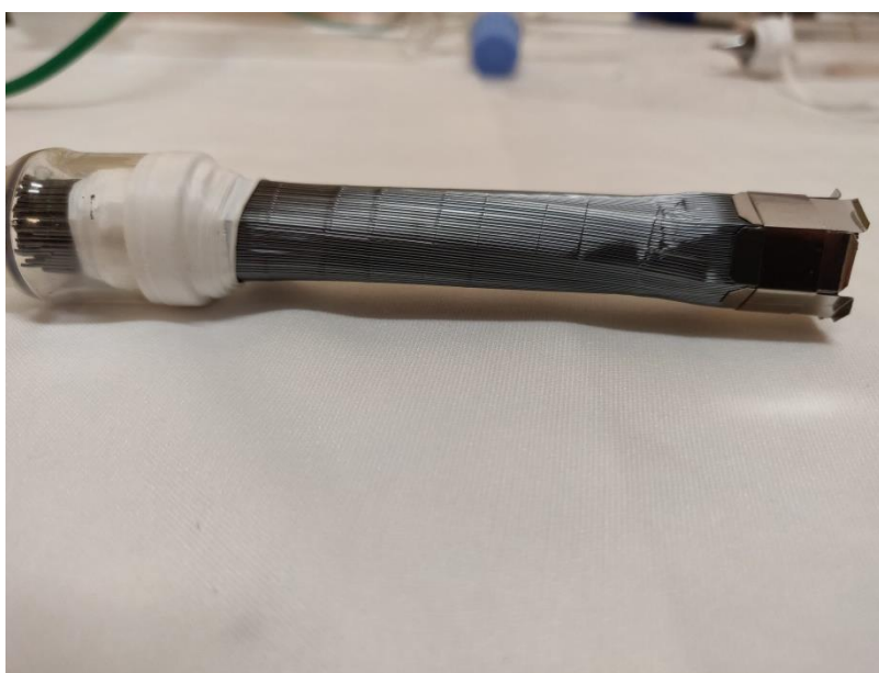
Figure 3.31 partially collapsed preform
