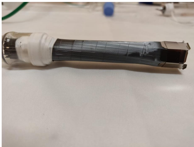
Figure 3.31 partially collapsed preform
