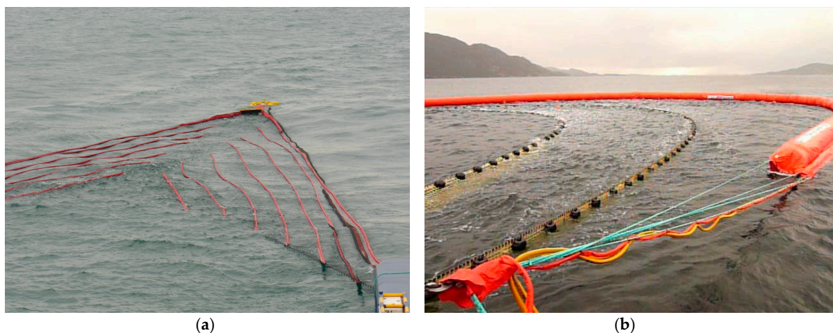
Figure 2. NOFO'2015 oil spill cleanup exercise: (a) MOS Sweeper and (b) DESMI Boom recovery systems tested on 9 June 2015 (photographs provided by NOFO).
