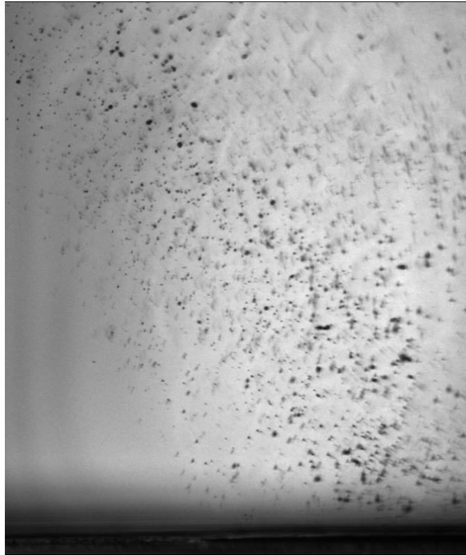
Figure 10.9: Image of the n-heptane spray obtained by Backlight Diffuse Illumination. The separation between the black zone at the bottom of the image and the grey background indicates z = 0 . The image size is 5.9 \times 5 \text{ mm}^2 with a spatial resolution of 2.3 \text{ }\mu\text{m}/\text{pixel} .
