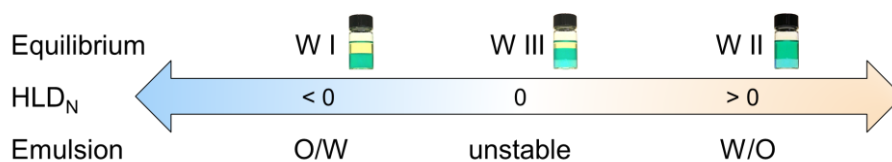
Figure 4.1. Illustration of SOW systems behaviour with HLD_N evolution when emulsified (top) and at equilibrium (bottom).
