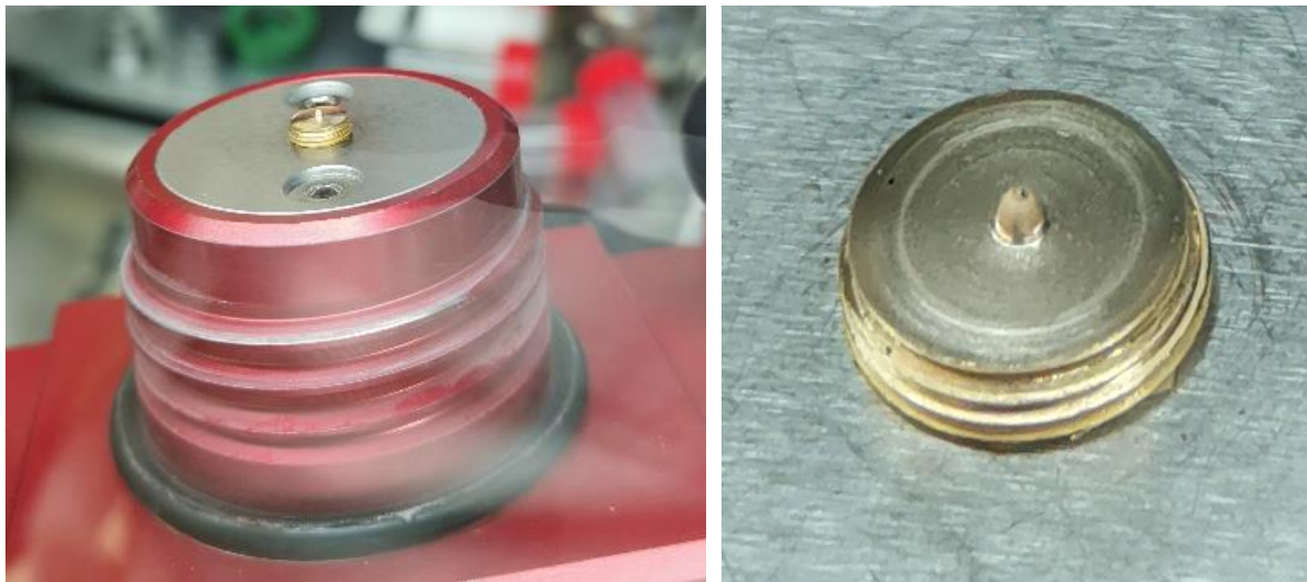
Figure 32: crucible photo after the DSC experiment (results in Figure 31)
