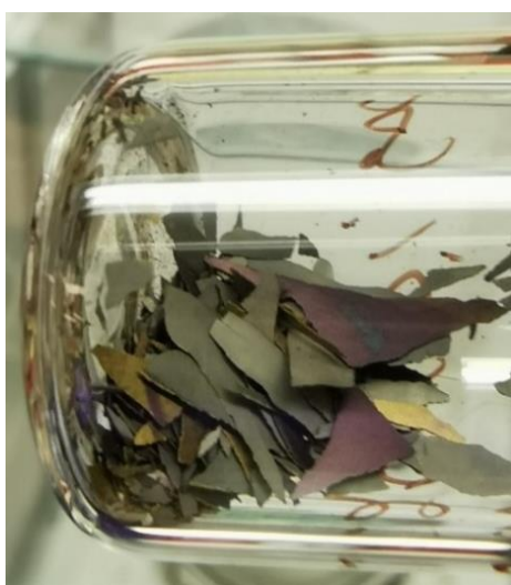
Figure 4: samples extracted from 28 days aged negative electrode at -20 °C
