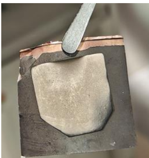
Figure 13: Photo of the obtained lithium deposit using the thermal evaporation technique
