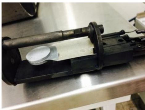
Figure 15 Sample installation for thermal conductivity measurement
