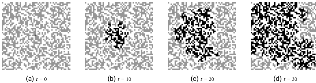
FIGURE 5.4. Example of the evolution of the trivial CA of fire propagation for a Moore neighbourhood with density d = 0.5 . The CA used is of size 50 \times 50 and state snapshots are taken every 10 iterations.
