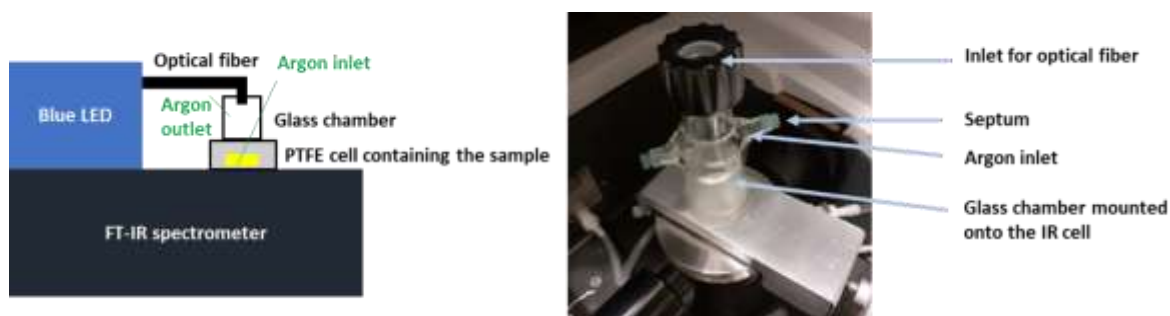
Figure S38 : Left: set-up used for the photoaccumulation-FTIR studies. Right: glass cell adapted by Bruno Coltrinari designed to work under an inert atmosphere.
