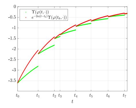
Figure 4.1: Time-evolution of the function  $\Upsilon(\varphi)$  along a trajectory of system (4.5) for the case described in Example 1 (green) and its upper bound in each sampling interval (red).
