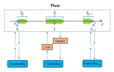
Figure 3.1: The system control setup.
