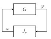
Figure 2.2: Alternative representation of the closed-loop system where G is a perturbed nominal control loop,  $\varphi$  is an auxiliary output representing the time derivative of the state between two sampling intervals,  $J_v$  is an integral operator and  $\omega$  is the sampling error.
