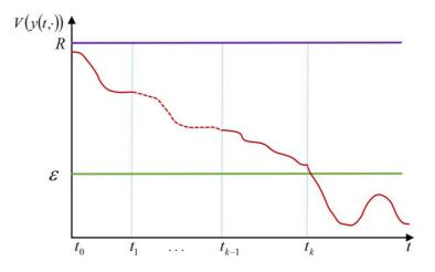
Figure 2.1: Schematic diagram of  $R\varepsilon$ -stability under Lyapunov method.
