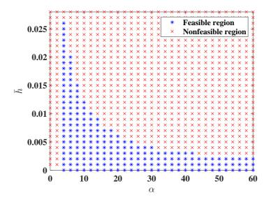
Figure 4.3: Influence of the estimate of the open-loop growth rate  $\alpha$  on the computation of the maximum allowable sampling interval  $\bar{h}$ . Feasible region (blue area) and non feasible region (red area) guaranteed by Theorem 4.1 with  $\mu = 10^{-5}$ .
