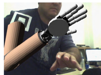
Figure 2.2: Example of partial avatarization. A user is augmented with a virtual prosthetic arm which he can see in AR. Figure extracted from the work of Lamounier Jr et al. (2012)
