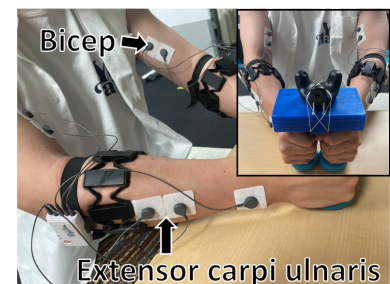
Figure 6.10: Physical task performed by the users to evaluate Proteus Effects: users had to grip these dumbbells while sEMG electrodes recorded their muscle activity.
