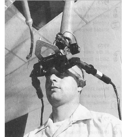
Figure 1.2: The "Sword of Damocles" (I. E. Sutherland, 1968). This AR device was released before even the invention of personal computers. Its nickname came from the fact that it was extremely heavy and needed to be suspended from the ceiling, above the user's head. Still regarded as a significant step in the development of AR, this work along with other pioneering contributions in computer graphics led Ivan Sutherland to receive the Turing Award in 1988.
