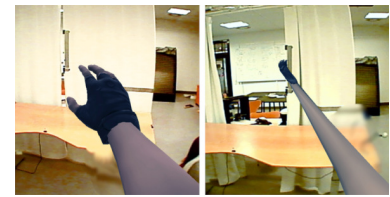
Figure 2.6: Example of partial avatarization with a VST HMD , borrowed from Feuchtner et al. (2017). Left: A virtual arm of normal length is embodied in first-person AR. Right: The user extends his virtual arm towards a normally unreachable (real) electric curtain and manipulates it.
