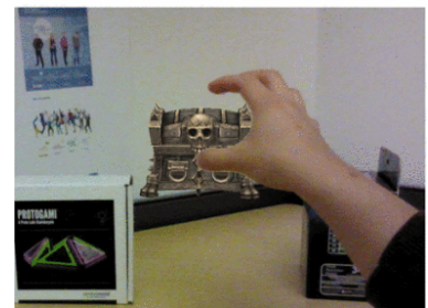
Figure 2.10: An illustration of virtual object rendering both with and without occlusion rendering. The lack of occlusion makes the user's hand appear behind the virtual chest (top), whereas it should normally appear in front of it (bottom). Figure extracted from Du et al. (2016).
