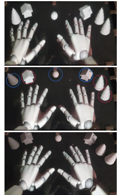
Figure 3.2: The experimental conditions from the participant’s point of view. Left The “VIRTUAL” condition where all the objects were virtual. Center The “MIXED” condition where there were both real and virtual objects mixed. Right The “REAL” condition where all objects were real. The 3D rendering allowed virtual objects to appear having the same 3D volume as their real counterparts.
