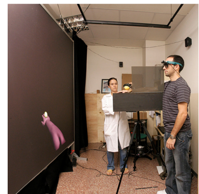
Figure 2.7: Example of partial avatarization with a CAVE system, borrowed from Slater (2008). The subject sees the virtual arm as projecting out of his right shoulder, while his own arm is hidden by a panel.
