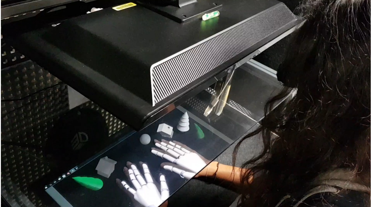
Figure 3.1: The experimental setup of our user study. A user is equipped with tracked shutter glasses and looks at her virtual hands under a semi-transparent mirror. The virtual hands are a reflection of the 3D screen hung above. The rendered perspective of the holograms is adapted to her point of view in real time. Part of the objects she sees is virtual (the green-colored ones).
