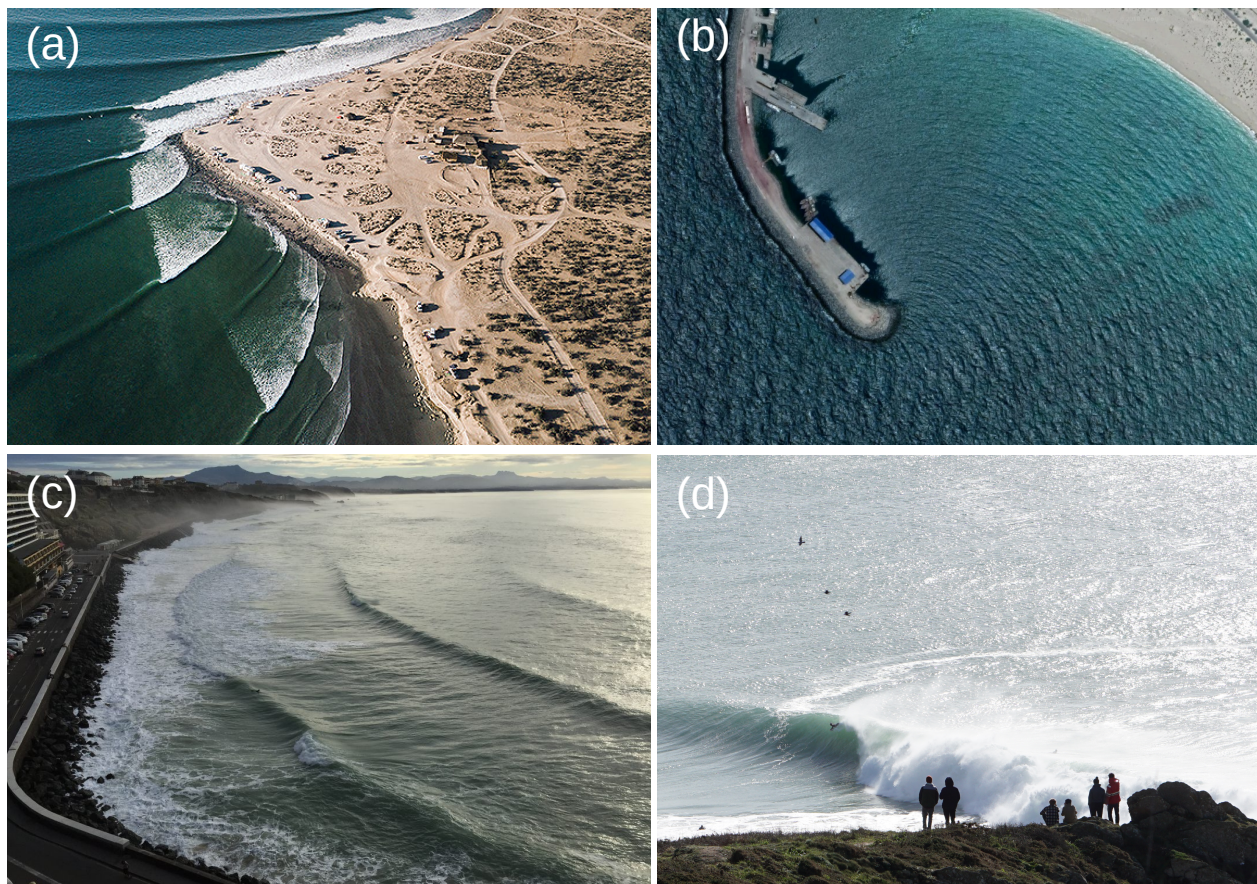
Figure 1.9: (a) Wave refraction around a headland, Scorpion Bay, Mexico. © Jacopo Cosmelli (b) Wave diffraction around the tip of a breakwater. Source : Google Earth (c) Wave shoaling at the Côte des Basques, Biarritz, France (d) Example of a plunging breaker in Brittany. © Tristan Keroullé.
