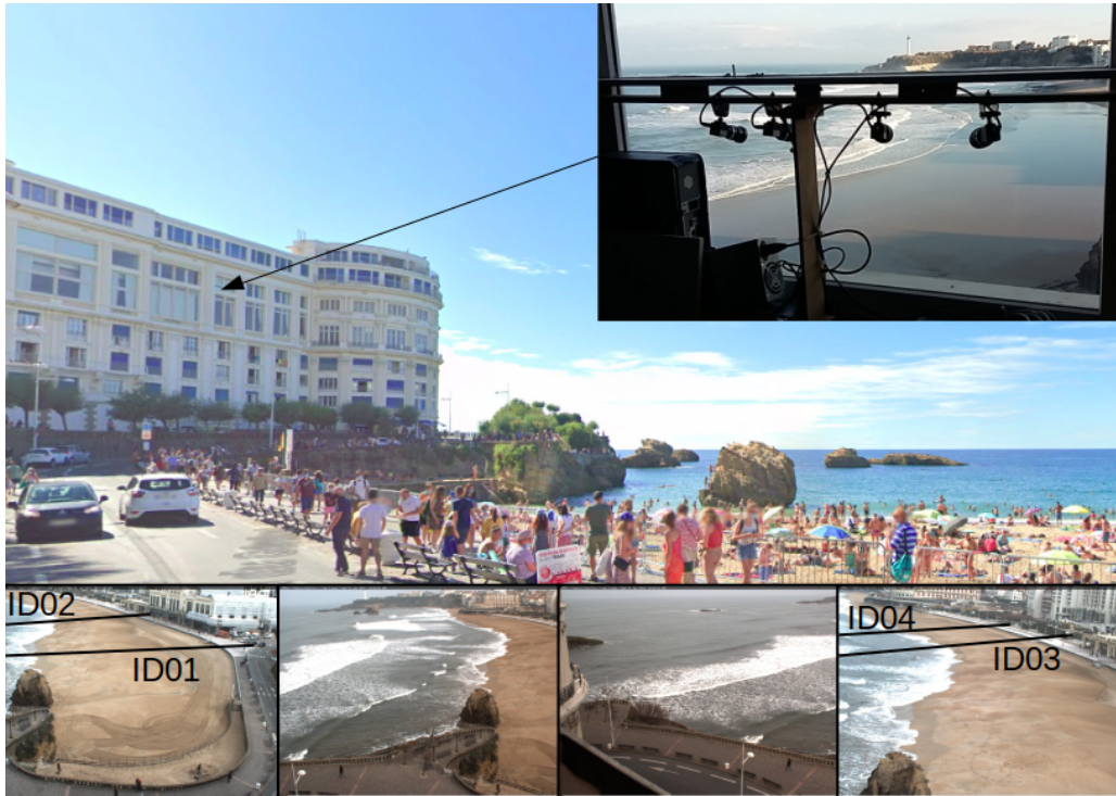
Figure 2.6: Video station of the GPB with black lines indicating the positions of cross-shore profiles where swash motion is followed.
