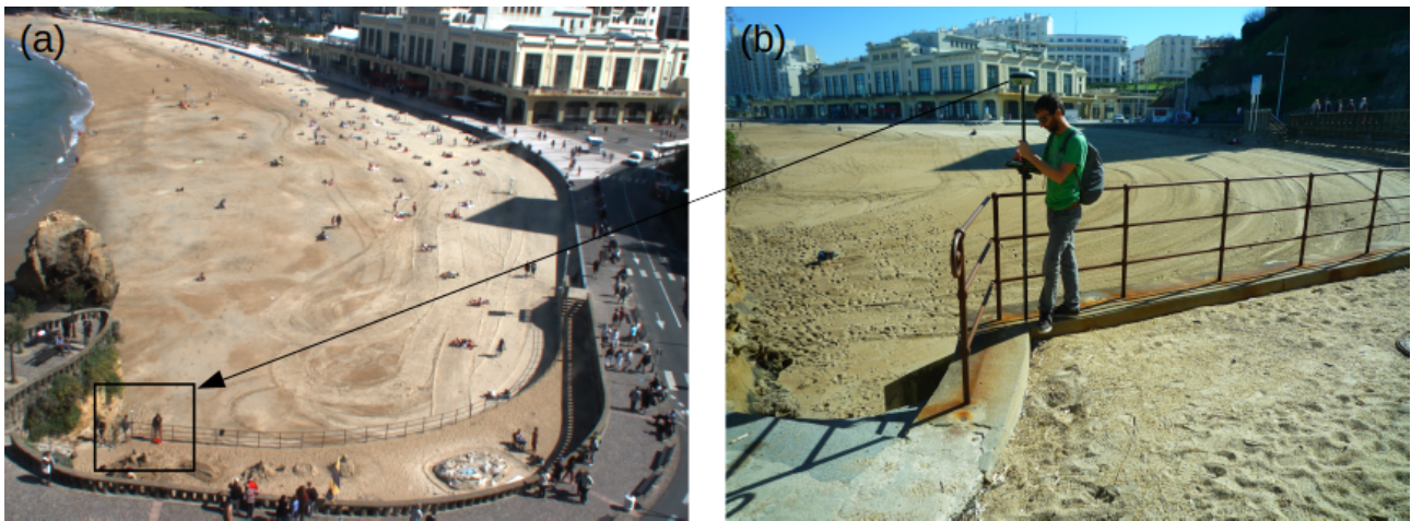
Figure 2.9: GCP pixel identification on the camera image (a) and DGPS-RTK measurement of the GCP coordinates (b).
