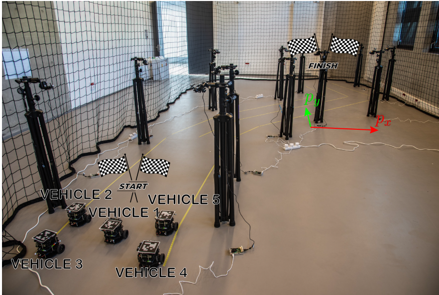
Figure 4.1: Experiment scenario setup: Multi-Vehicle System with 5 vehicles in the starting place and Sensor Network composed of 12 cameras and Raspberry PI computers.
